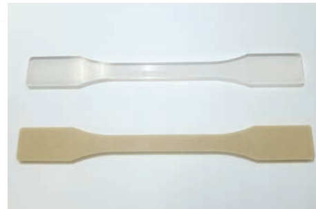
Examples of molded items (Top: Polylactic acid only; bottom: polylactic acid combined with pulp)
