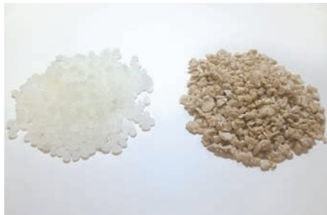
Plastic pellets (Left: Polylactic acid only; right: polylactic acid combined with pulp)
