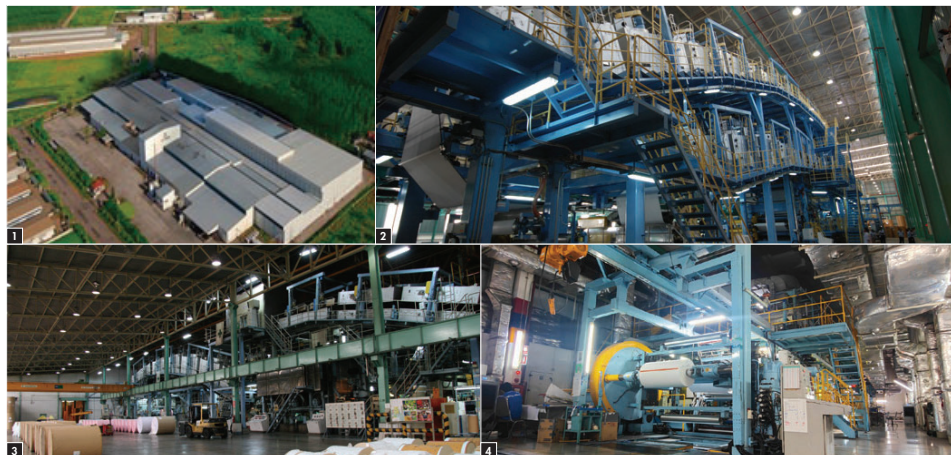
1 Panoramic view of the Prachinburi Mill 2 A thermal paper coater (CM2) 3 A carbonless paper coater (CM1) 4 An adhesive paper laminator (LM2/OLT)
