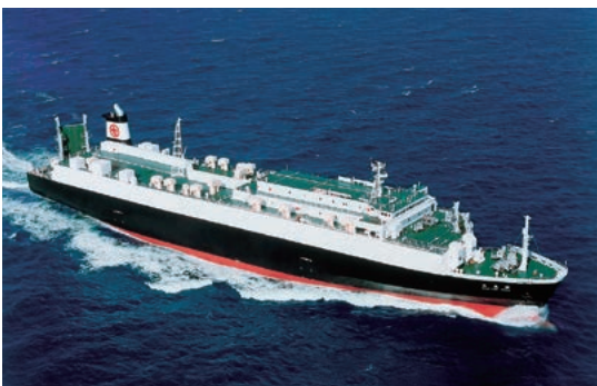
Roll-on roll-off ship that can deliver vehicles carrying goods
