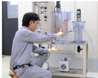
Laboratory testing apparatus for biological treatment
