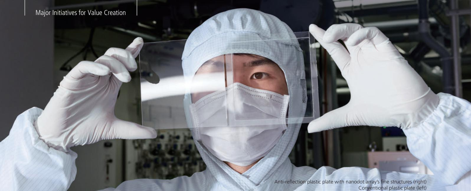
Anti-reflection plastic plate with nanodot array's fine structures (right)
