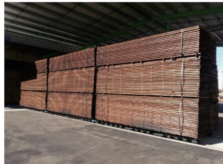
TMT that is processed with high temperature in the special kiln
