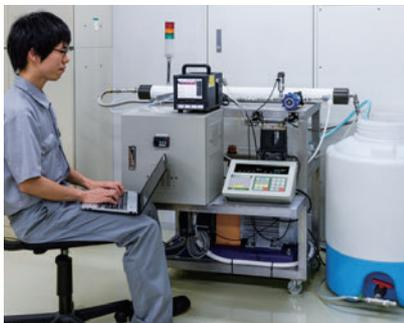
Laboratory testing apparatus for membrane treatment
