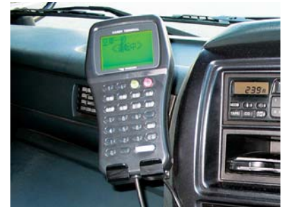
Photo 2 A digital tachograph like the ones installed in our entire vehicle fleet to collect driving data.
