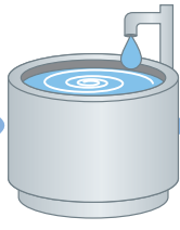
Pulping Recovered paper is broken down in water.
