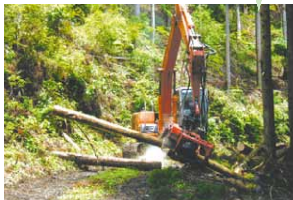
After being downed by a chainsaw, trees are cut into predetermined lengths using heavy machinery.
