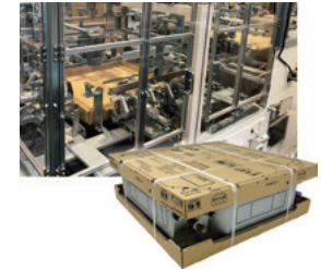
The packaging tray and auto-assemble machinery for large commercial-use air conditioner developed together with Daikin Industries, Ltd.
