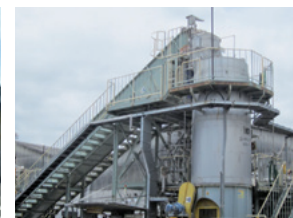
Kneading pulper, dissolving equipment for difficult-to-recycling paper (Oji Materia Fuji Mill)
