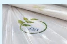
Succeeded in developing an eco-friendly biaxially stretched polypropylene film that contains polylactic acid. (P37)
