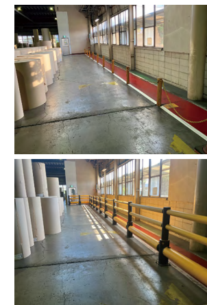
Installation of safety fences around pathways in plants (Above: before installation; Below: after installation)
