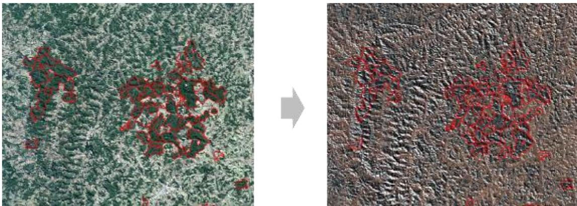
Figure 5.2 Topographic correction of satellite images (left: before correction, right: after correction)
